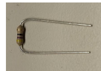
Figure 3. Form the leads of the resistor as shown
