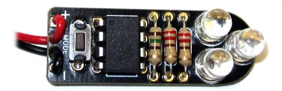
Your Lux Spectralis 2 kit is now complete! Replace the batteries and turn on the power switch. Use the "MODE" button to advance through the pre-programmed color patterns. Enjoy!
