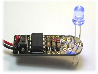
Test each LED and identify its color. The LED should light up. If not, try one of the other LED locations. Once all the LEDs are identified, turn the power off using the power switch or remove the batteries from the battery holder.
