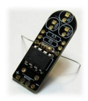
Repeat for R2 (green LED resistor) and R3 (blue LED resistor). These are 1/4W 220 ohm resistors, marked with red, red, brown and gold stripes.
