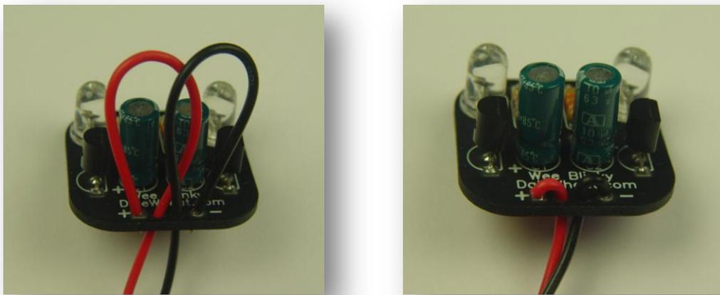
Photo 21. Lace the power wires for strain relief.
