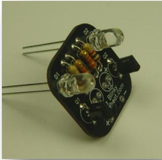
Photo 14. LEDs inserted flush against PCB.
