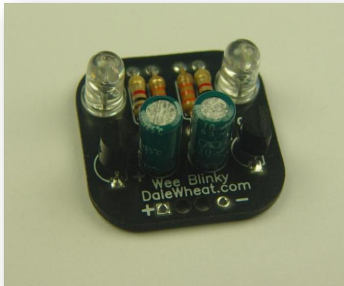
Photo 20. The right way to install the capacitors.
