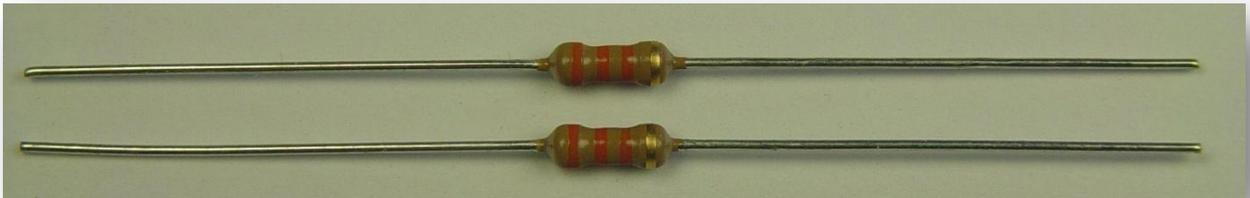
Photo 3. Resistors R2 and R3 are  $33\text{K}\Omega$  (thirty three thousand ohms), with three orange stripes.
