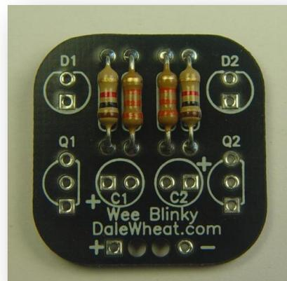
Photo 7. The correct way to install the resistors.
