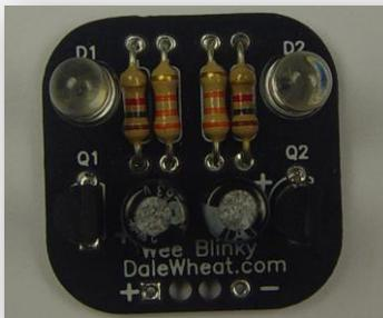
Photo 1: A properly assembled Wee Blinky
