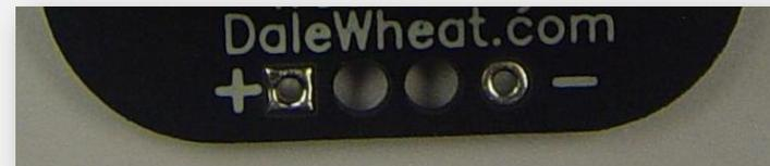
Photo 2: Power connection points for the Wee Blinky.
