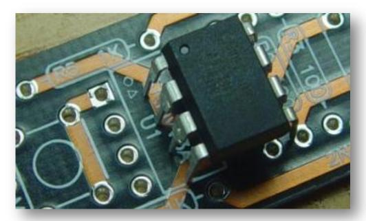
Make sure all eight (8) pins of the computer chip are inserted into their holes by looking at the back side of the PCB and counting how many little legs are poking through. A couple of them may be bent
